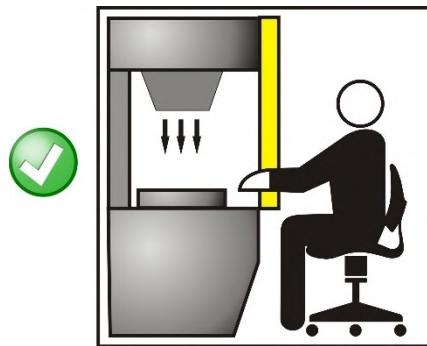
Fig 10 - Correct light curtain positioning
