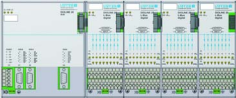
Fig. 3: MVB Buscoupler with I/O Modules
