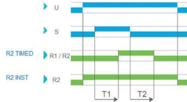
Function Ac - On/Off Delay (Delay on make/break)
