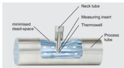
The patented hygienic design of the TW61 flow-through housing enables dead-space minimised, invasive temperature measurement and a flexible mounting position through self-draining.
