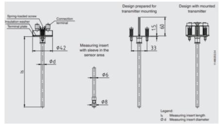
Neck tube per DIN 43772, straight, with/without compression fitting
